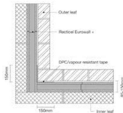
**Fig. 7. Internal corner, or external corner with mitred board joints**
